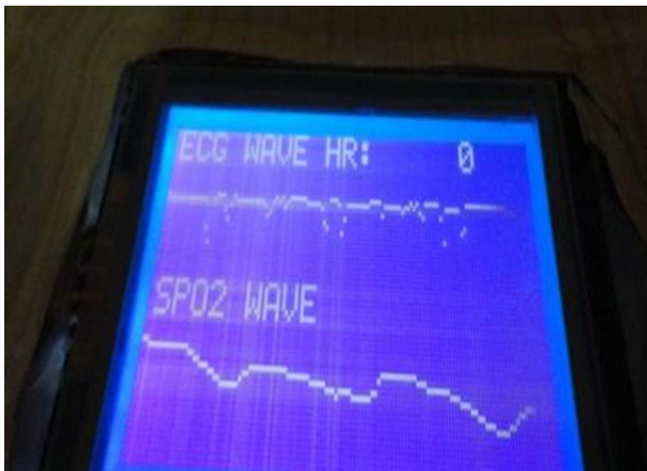
Figure 7.3. ECG and saturated oxygen signals plotted on a GLCD display.
